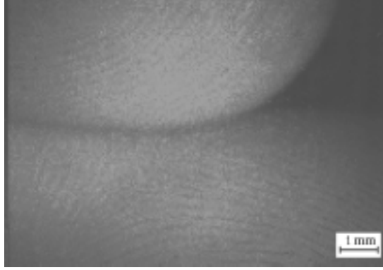
Fig. 5. Biospeckle-field sample recorded by means of a CCD-camera. The size of the investigated field is 2 \times 2 \text{ mm}^2 and the spatial resolution is 768 \times 494 points.
